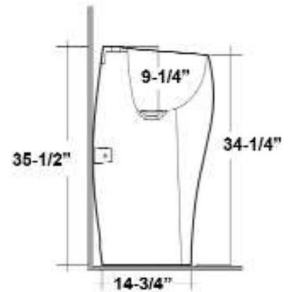
Dimensions of fixture are nominal and may vary within the range of tolerances established by ASME Standard A112.19.2-13. Dimensions and specifications subject to change without notice.
