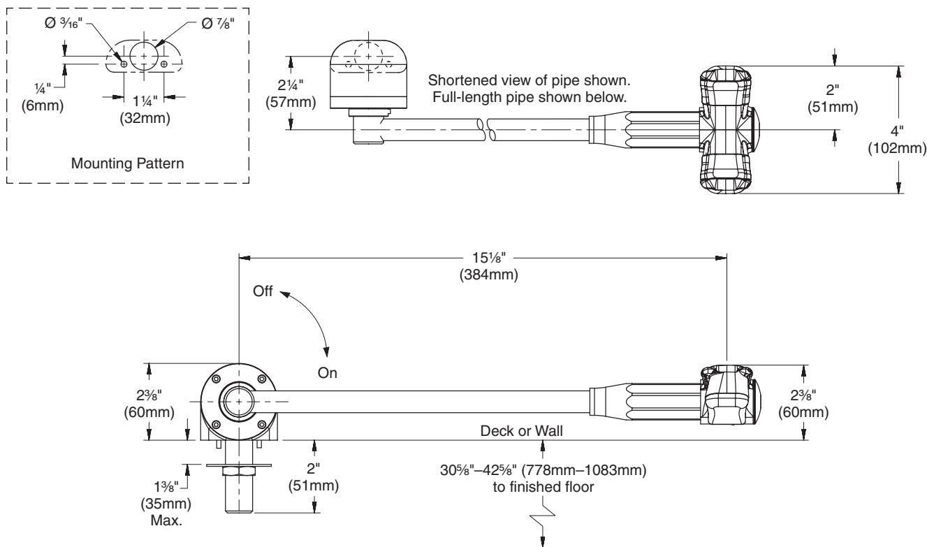
**Dimensions — S19-290D, S19-290W** (deck-mounted unit shown)
