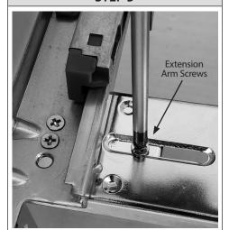
Tighten Extension Arms Screws (D) at desired location.
