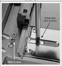
Remove the Extension Arm Screws (D) and loosen the Slide Mounting Screws (E) from slides.
