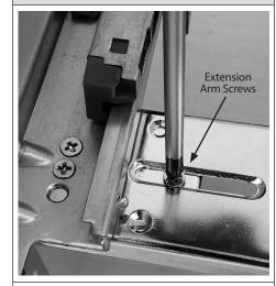
Loosen the Extension Arm Screws (D).
