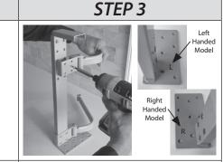
Install both Corner Support Arms to the Corner Support as show above with four (4) #10 x 5/8" washer head machine screws per arm and tighten securely. The Corner Support is marked with an L for left handed models and an R for right-handed models.
