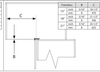
Using the chart and diagram, with tape measure and square, lightly mark mounting locations inside the cabinet for the appropriate tray size ordered. For face-framed cabinets the supports are designed to be pulled up tight behind the face-frame.
