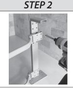
Install both Center Support Arms to the Center Support as show above with (4) #10 x 5/8" washer head machine screws per arm and tighten securely. The upper shelf has three possible shelf heights, make note of your selection and match it in step 3.
