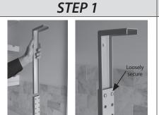
Slide both of the Telescopic Support Extensions into the top of the Center Support and Corner Support. Loosely secure in top two holes with (2) #10 x 5/8" washer head machine screws per support.
