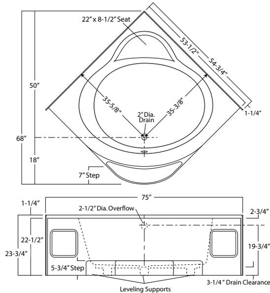
**Illustration 1b - Unit Dimension & Alcove Framing Guidelines (dimensional tolerance +0 / -3/8")**
