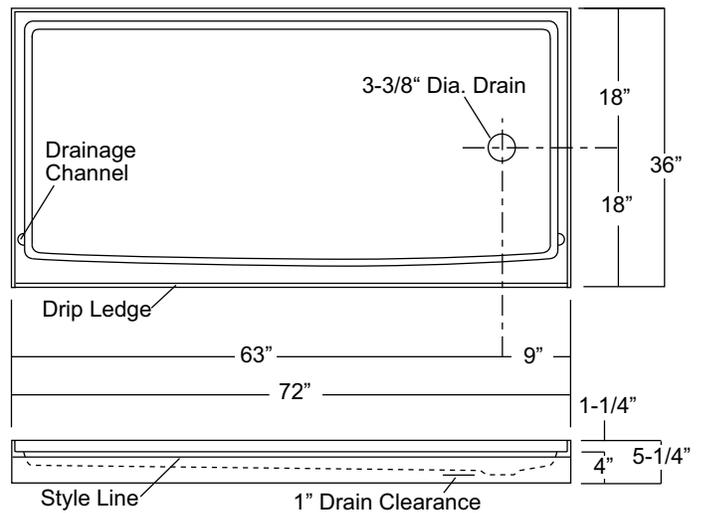
**NOTE:** Critical enclosure dimensions should be taken directly from the installed shower base with finished wall surround.
