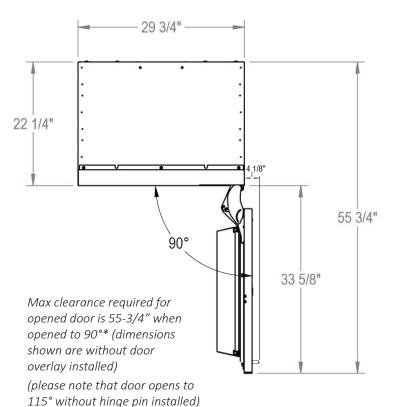
PLEASE NOTE: When installing column adjacent to wall, a 2" clearance is required if door opens towards the wall \*90° achieved when included hinge stop pin is installed. Pin must be installed prior to full integration
