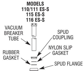
**B** Insert Tube into Fixture Spud.
