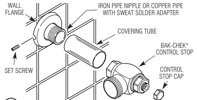
**D** Tighten Wall Flange Set Screw with hex wrench supplied. **DO NOT** install Vandal Resistant Stop Cap at this time.
