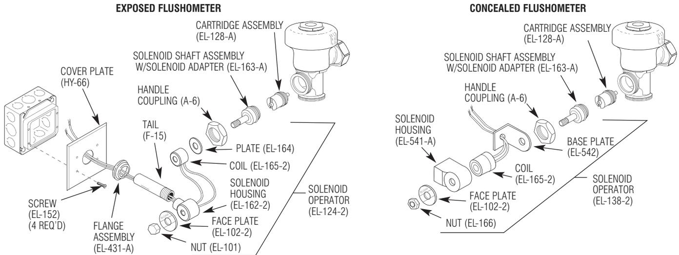
**Important:** Do not remove coil from solenoid plunger guide unless power has been disconnected. Failure to do so may damage sensor, coil and transformer.
