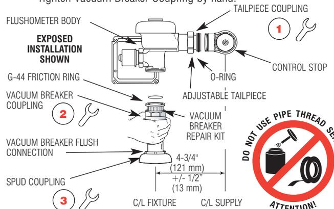
**C** Align Flushometer Body and securely tighten first the Tailpiece Coupling (1), then the Vacuum Breaker and Pipe Couplings (2), and finally the Spud Coupling (3). Use a wrench to tighten these couplings in the order shown.
