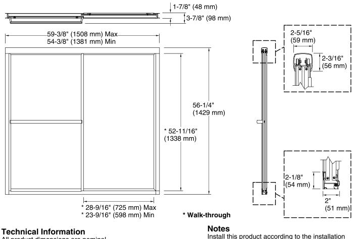
All product dimensions are nominal.Installation type:For bath installationOpening Width - Min:54-3/8" (1381 mm)Opening Width - Max:59-3/8" (1508 mm)Walk-through - Min:23-9/16" (599 mm)Walk-through - Max:28-9/16" (726 mm)Glass thickness:1/8" (3 mm)
