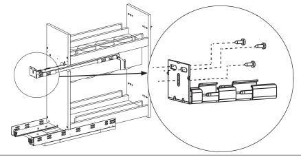
Remove the unit from the base again and then slide the rear mounting bracket off the slide. Align the rear bracket prongs with the indentation marks on the rear of the cabinet and secure with three (3)  $\#8 \times 5/8$ " Pan Head Wood Screws in the slots as shown. Re-install the unit onto the slides, making sure as you push it in the cabinet, that the top slide is properly seated into the rear mounting bracket. Operate the unit to make sure the undermount slides are working properly.
