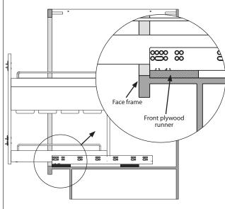
Remove the base from the unit by releasing the slide clips. In framed cabinets, center the unit in the opening making sure the front plywood runner is pulled tight against the back of the face frame. For frameless cabinets, place the unit within 1-1/2" of the left of the cabinet and the front plywood runner needs to be set back 3/4". Install with the four (4) #10 x 3/4" Pan Head Wood Screws provided in the four pre-drilled holes in the runners. Re-install the unit onto the slides.
