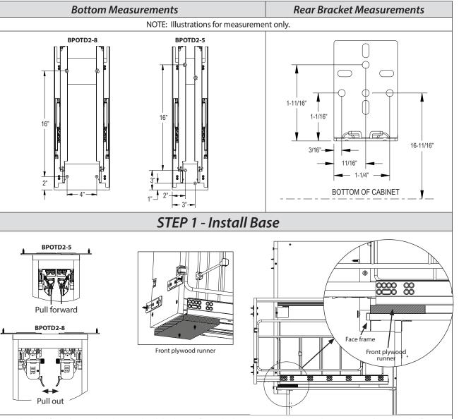
Remove the base from the unit by releasing the slide clips. In framed cabinets, center the unit in the opening making sure the front plywood runner is pulled tight against the back of the face frame. For frameless cabinets, place the unit within 1-1/2" of the left of the cabinet and the front plywood runner needs to be set back 3/4". Install with the four (4) #10 x 3/4" Pan Head Wood Screws provided in the four pre-drilled holes in the runners.
