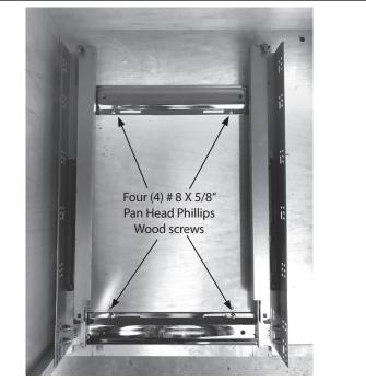
Place the slide base inside the cabinet, pulling the front cross member tight against the rear of the face frame. For frameless cabinets, set the front cross member back 3/4". For inset door applications, slide the base back from the above measurements plus the thickness of the door. Firmly secure with four (4) # 8 X 5/8" Pan Head Phillips Wood screws provided in the locations shown above.
