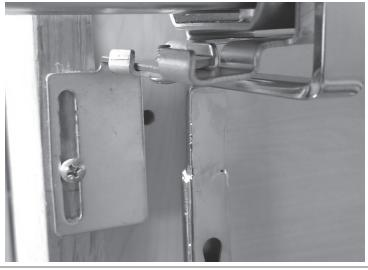
Pull the top front mounting bracket into position on the side of the face frame (or cabinet) allowing for a 3/16" setback (shown left above). Firmly secure with one (1) #8 x 5/8" Pan Head Wood Screw. Make sure the gap between the unit and the side of the face frame is equal from top to bottom. Adjust accordingly and then securely tighten the bracket set screw (shown right above). Operate the unit and make adjustments as necessary for the slides to operate smoothly.
