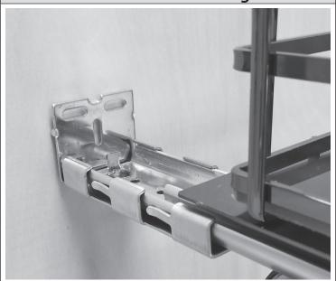
If the countertop is installed, pull the organizer partially open to gain access to the upper slide. Firmly grasping the upper slide, tap it against the back of the cabinet. The rear bracket should make small indentations in the back of the cabinet. Proceed to step 4. If countertop is not installed, pull the organizer partially out to gain access to the rear bracket and install three (3) #8 x 5/8" Pan Head Wood Screws provided in the slots. Proceed to step 5.
