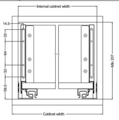
Install the front mounting brackets on the front using the screws provided and according to the dimensions above.
