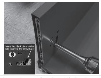
Use a screwdriver to turn the mechanism in the drawer box that will release the mounting brackets that are on the inside.
