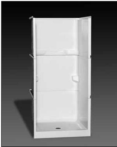
**Specification** – Oasis 3-piece FRP gelcoat shower compartment, SH3P-3636, offered in a standard 4-inch or 6-inch (ABF) dam configuration. ActivLife package includes factory-applied reinforcement, in compliance with HUD/FHA Fair Housing Act Design Manual, shall include back wall and both side wall reinforcement for horizontal bar application.
