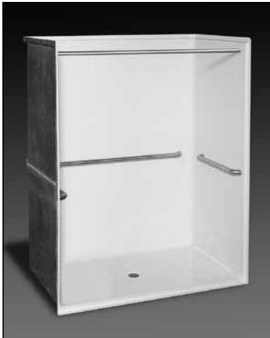
**Specification** – Oasis one-piece FRP gelcoat shower compartment SHFW-6235, having a 60 x 30-inch minimum clear interior dimension and ½-inch high maximum finished threshold with floor attachment flange on lower threshold. A factory-equipped package, in compliance with 2010 ADA Standards & ICC/ANSI A117.1-2009 for Accessible Design, shall include a horizontal bar across each side wall and back wall and shower curtain rod.
