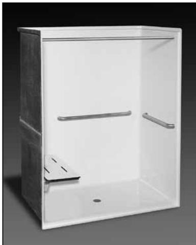
**Specification** – Oasis one-piece FRP gelcoat shower compartment SHFW-6235, having a 60 x 30-inch minimum clear interior dimension and ½-inch high maximum finished threshold with floor attachment flange on lower threshold. A factory-equipped package, in compliance with 2010 ADA Standards & ICC/ANSI A117.1-2009 for Accessible Design, shall include a horizontal bar across the side wall opposite the seat wall and back wall, a folding seat, and shower curtain rod.
