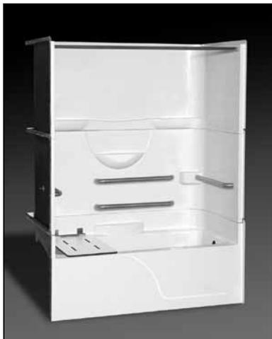
**Specification** – Oasis 3-piece, 60 x 30-inch deep, FRP gelcoat bathtub model TS3P-6030 ABF (17.25-inch apron) having a factory-equipped package in compliance with 2010 ADA Standards for Accessible Design. Package includes 2-horizontal bars on back wall, single horizontal bar on head end wall, horizontal bar on control wall, pivot-hinge FOLDING in-tub seat at head end and shower curtain rod.
